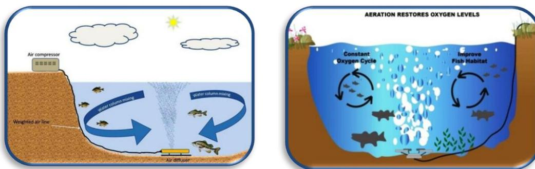
Figure (7): Artificial Aeration System ([www.Watgardengems.com](http://www.Watgardengems.com))
