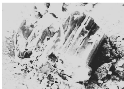
Fig. (2): SEM shows microcracks with Basalt texture, pitting crystal, can be noted.
