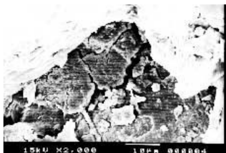
Fig. (5): SEM shows an intermineral network of fissures and the deformation of minerals
