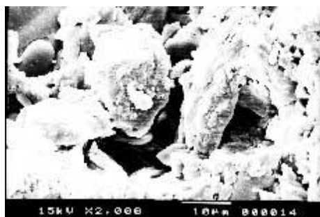
Fig. (1) : SEM shows the dislocation and the separation of the grains and the formation of residual pores.
