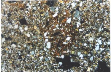
Photo (3): Silasepic plasma fabric, with frequent silt-sized quartz particles ( sub-surface of profile 1, CN. 25X)
