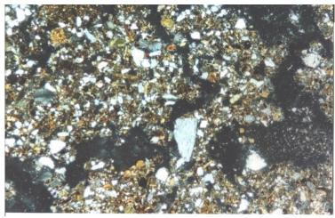
Photo (1): Porphyroskelic plasmic fabric with interconnected irregular orthovughs, channels and chambers (surface of profile 1, CN. 25X).
