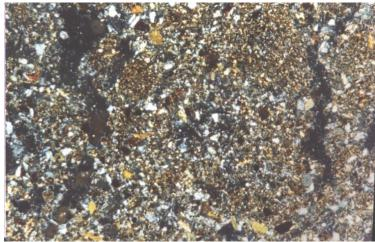
Photo (8): Dense plasma with silty sized grains, subparallel grains insepic and fine argillaceous nodules (sub-surface of profile 4, CN. 50X).
