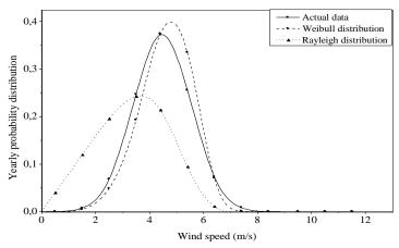
Fig. (6): Weibull and Rayleigh approximations of the actual probability distribution of wind speeds
