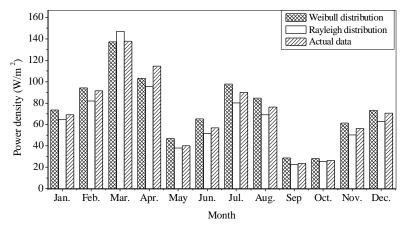
Fig. (8): Wind power density obtained from the actual data versus those obtained from the Weibull and Rayleigh models on a monthly basis.
