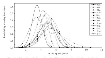
Fig. (2): Monthly wind speed probability density distributions derived from the measured data of Taiz for whole years
