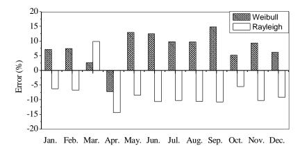
Fig. (9): Error values in calculating the wind power density on monthly basis obtained from the Weibull and Rayleigh models in reference to the wind power density obtained from the measured data
